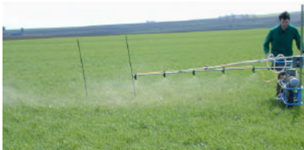
Fig.1: Application with a Schachtner plot sprayer, wind speed 7 m/s. XR 110 02, 1.9 bar, 200 l/ha
